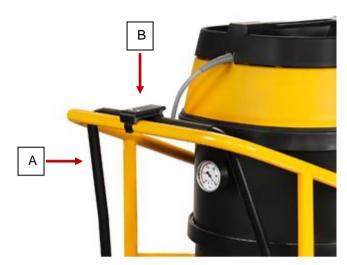
It is possible to lift the front nozzle from the floor by pulling the black handle [A] near the steering grip.
